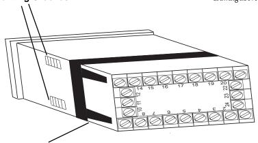
the tabs on the bracket arm are seated in the mounting grooves on the side of the unit.
